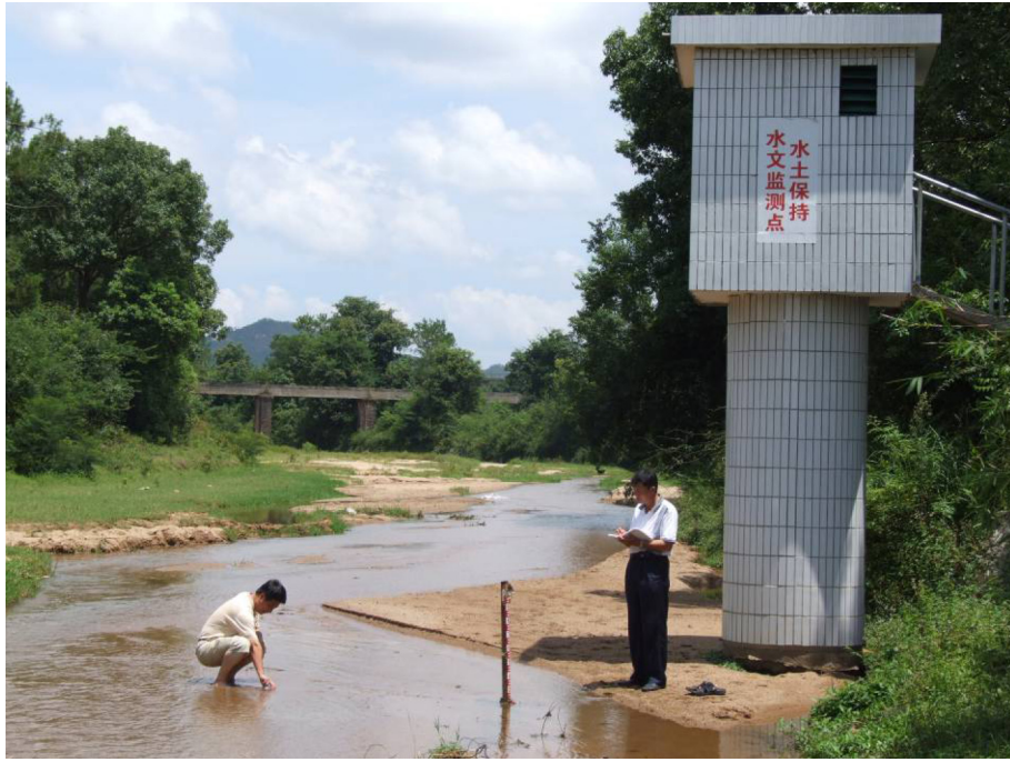
Fig. S8. The quantity of run-off and water samples to detect soil erosion were measured every 2 and 12 h, respectively, downstream of the project area.
